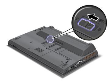
4. Press the latch as shown in the illustration below and detach the battery.
